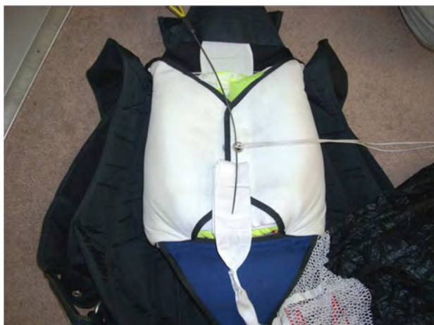
“S”-fold the remaining Bridle as shown.
