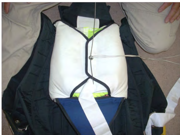
Close the side flaps. Secure with a temporary pin.
