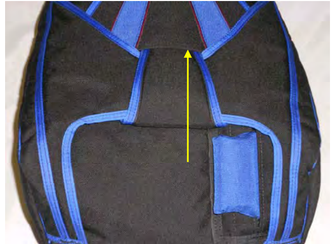
Close the Main Pin Protector Flap.
