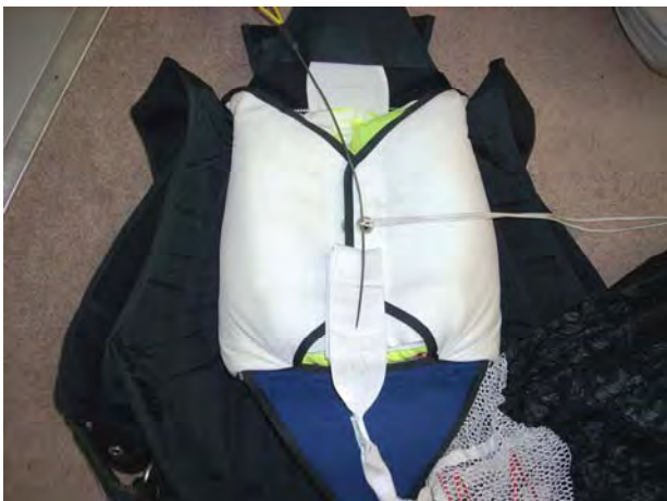
“S”-fold the remaining Bridle as shown.
