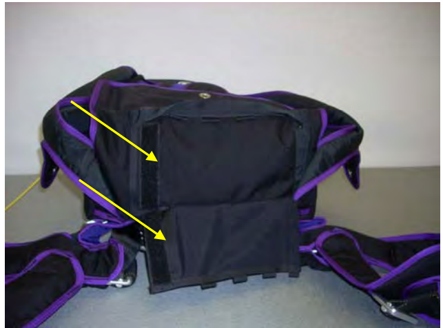
The AFF Left Side Main Deployment Pouch before assembly of the Handle.
