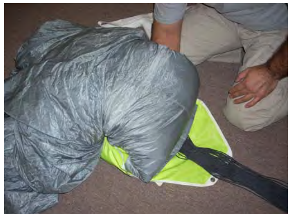
"S"-fold the canopy over onto itself once again.
