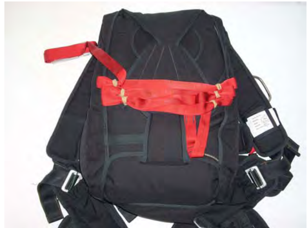
Continue stowing until last rubber band.
