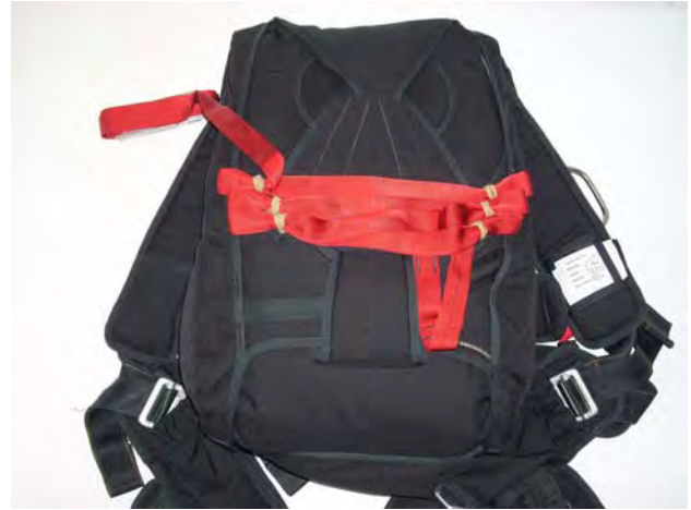
Continue stowing until last rubber band.
