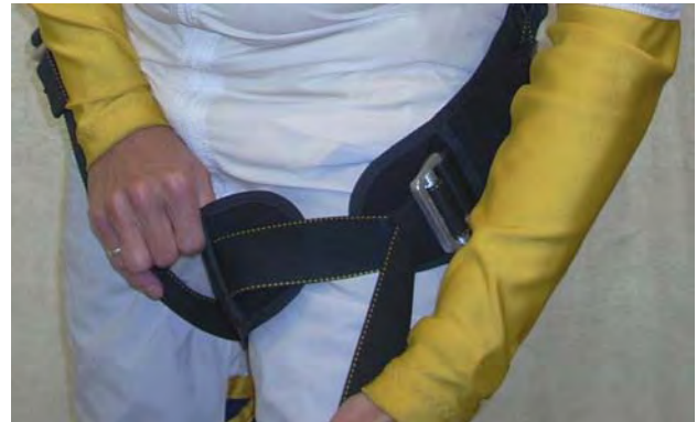
Adjusting the Leg Straps.
