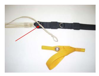
Pass the Steering Line through the appropriate Slider Grommet then through the mini ring closest to the lines.
