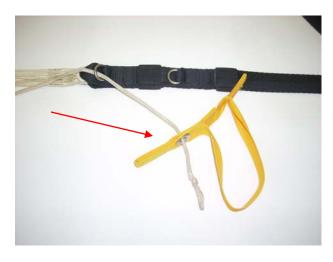
Pass the Steering Line through the rear of the Steering Toggle.
