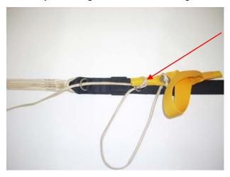
Pass the Steering Toggle through the "cat's eye" of the steering line to secure the line.
