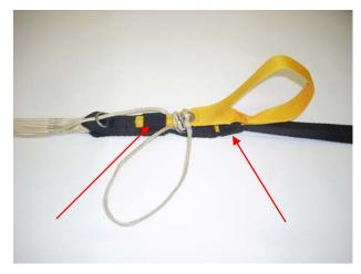
Stow the Toggle Tabs under the elastic keepers on the risers.
