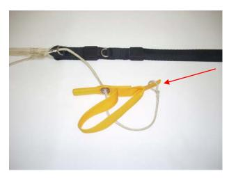
Slip the loop of the Steering Line over the lower tab of the Steering Toggle.
