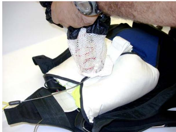
Thread a pull-up cord through the Reserve Pilot-chute and center over the side flap grommets.
